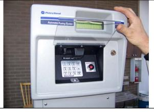
Lift associated pump nozzle for fuel selected and push the silver lever down to start the fuel pump.
